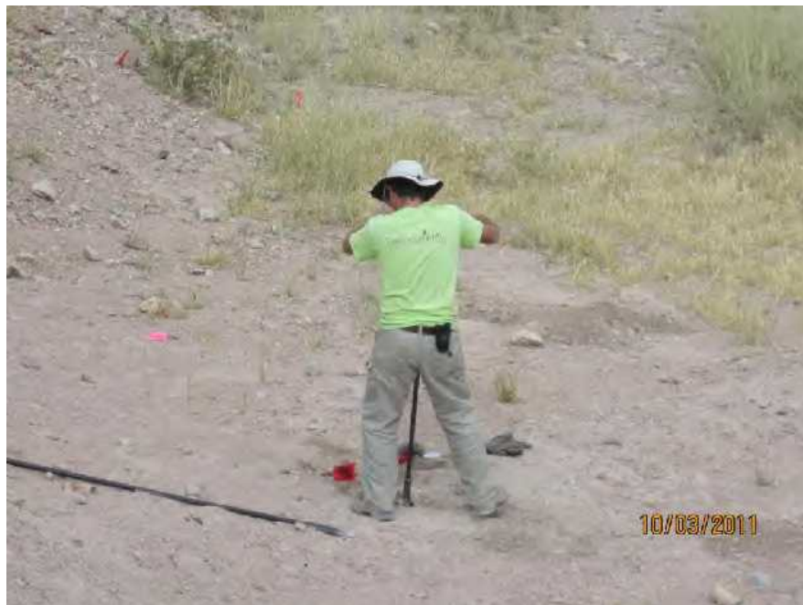
Photo 8 TPMC Technician Collecting Soil Sample
