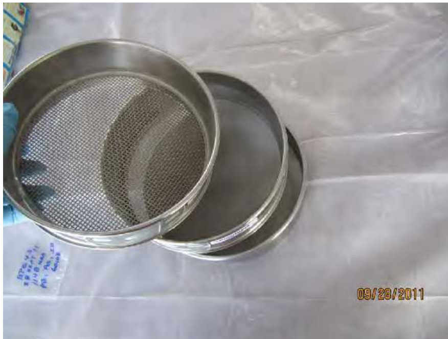
Photo 10 #8-Size Sieves used to segregate Fine Soils from Coarse Material and Bullet Fragments
