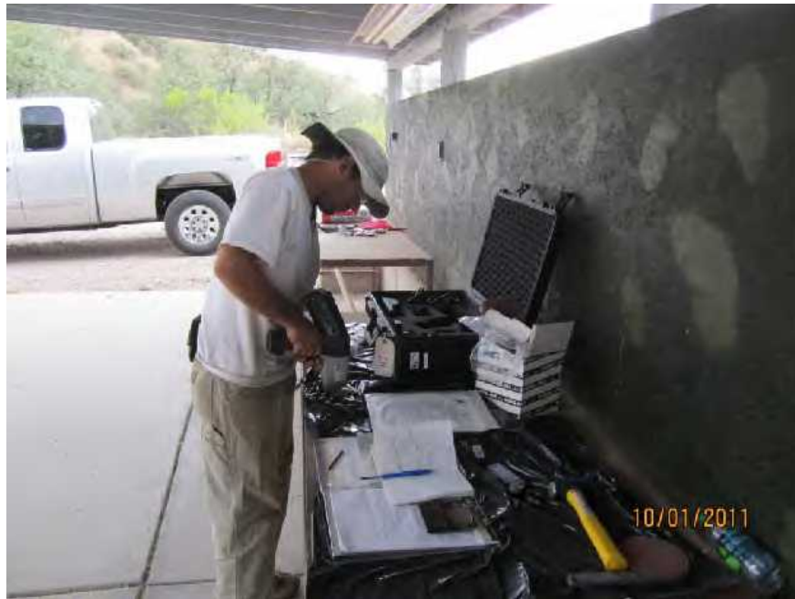
Photo 9 TPMC Technician Screening Soil Sample with X-Ray Fluorescence Instrument
